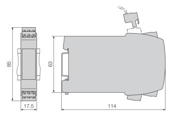
Fig. 12. SINEAX V 624 in housing **P12/17 St** clipped onto a rail «G» ( $35 \times 15$  mm or  $35 \times 7.5$  mm, acc. to EN 50 022), screw terminals pluggable.
