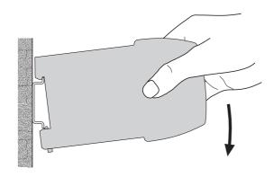
Fig. 3. Mounting onto top-hat rails  $35 \times 15$  or  $35 \times 7.5$  mm.
