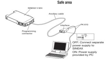
Fig. 6. Configuring a SINEAX V 624 without the power supply. For this case the switch on the interface must be set to "ON".
